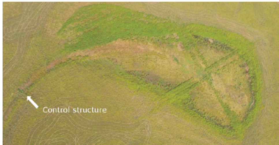
A 3.5-acre temporary/seasonal wetland within field T5. The wetland drains to the left (west) of the photo. Near the left edge of the photo is a green line running perpendicular to the drainage. This is the control structure used to regulate water depth in the wetland. This wetland was planted to two varieties of prairie cordgrass by direct seeding or by transplanting. The experimental cordgrass transects form a green "X" centered on the deepest part of the wetland. A green ring of cordgrass is also visible around the wetland edge—this was grown for seed production and was not part of the experiment. Adapted from Zilverberg et al. (2014a).
